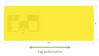
The label is delivered with no adhesive on the backside, so additional adhesive or plastic pockets are required for label attachment.
